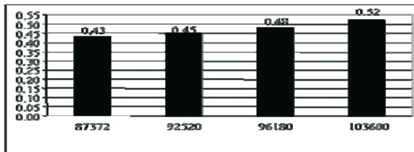
Fig. 19. Smoking of engine fumes depending on the km run
