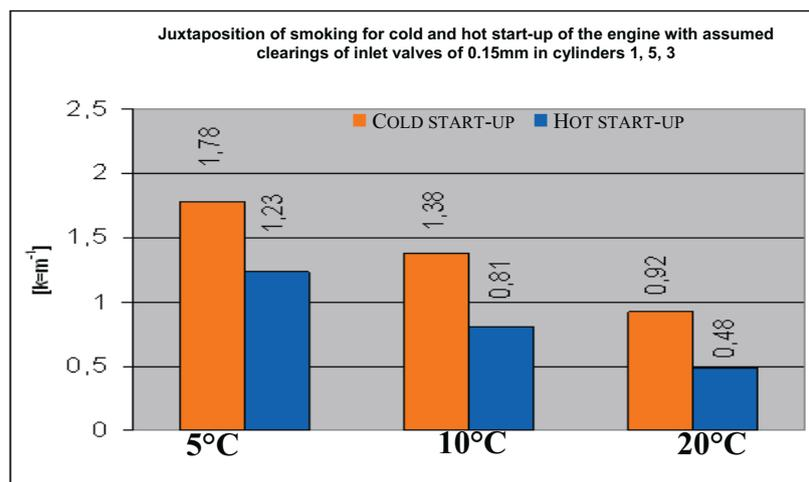
Fig. 15. Juxtaposition of smoking for cold and hot start-up of the engine with assumed clearings of inlet valves of 0.15 mm in cylinders 1, 5, 3
