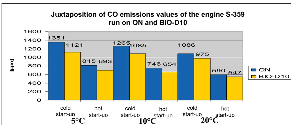
Fig. 20. Juxtaposition of CO emissions values of the engine S-359 run on ON and BIO-D10
