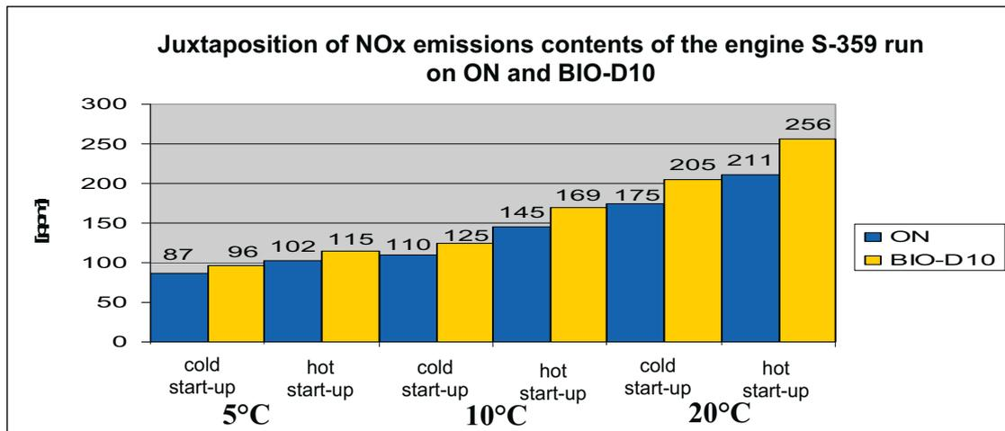
Fig. 22. Juxtaposition of NO<sub>x</sub> emissions contents of the engine S-359 run on ON and BIO-D10
