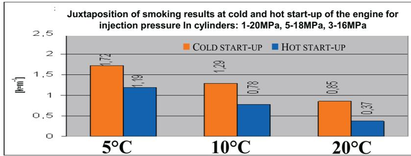
Fig. 11. Juxtaposition of smoking results at cold and hot start-up of the engine for injection pressure In cylinders: 1-20 MPa, 5-18 MPa, 3-16 MPa
