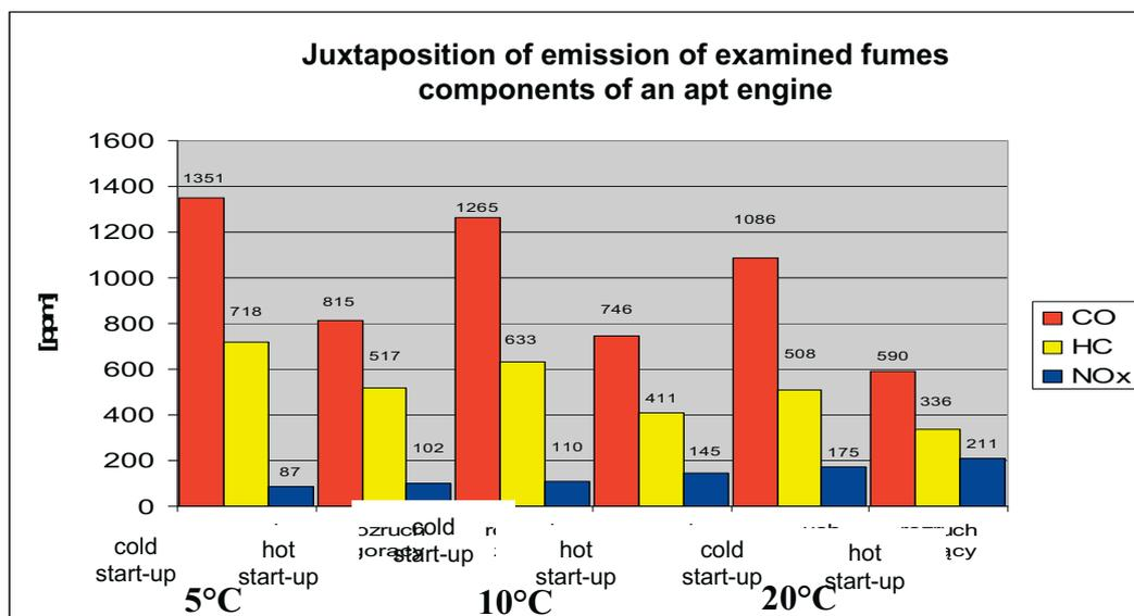
Fig. 5. Juxtaposition of emission of examined fumes components of an apt engine
