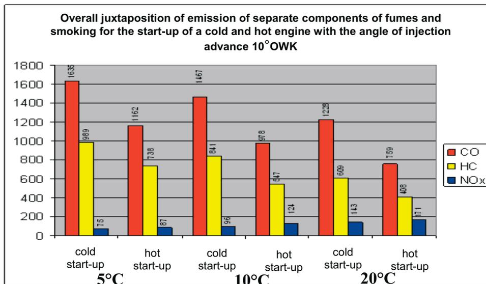
Fig. 6. Overall juxtaposition of emission of separate components of fumes and smoking for the start-up of a cold and hot engine with the angle of injection advance 10°OWK
