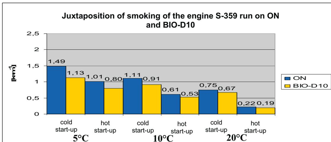
Fig. 23. Juxtaposition of smoking of the engine S-359 run on ON and BIO-D10
