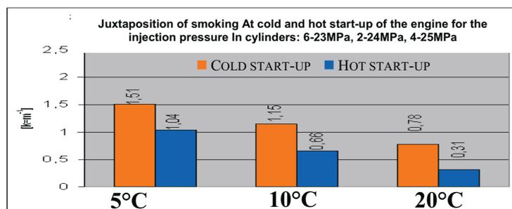
Fig. 13. Juxtaposition of smoking At cold and hot start-up of the engine for the injection pressure In cylinders: 6-23 MPa, 2-24 MPa, 4-25 MPa
