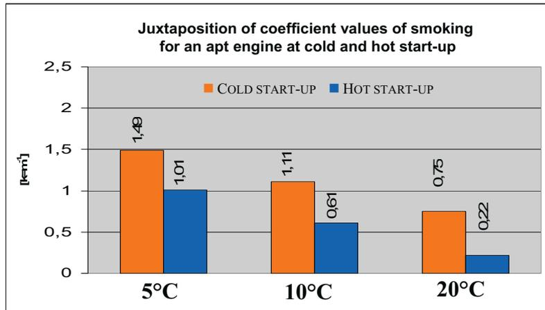
Fig. 6. Juxtaposition of coefficient values of smoking for an apt engine at cold and hot start-up
