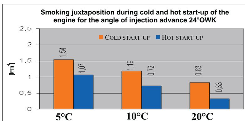
Fig. 9. Smoking juxtaposition during cold and hot start-up of the engine for the angle of injection advance 24°OWK
