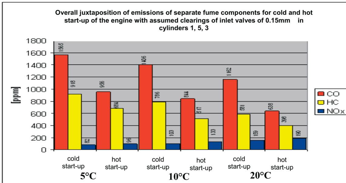
Fig. 14. Overall juxtaposition of emissions of separate fume components for cold and hot start-up of the engine with assumed clearings of inlet valves of 0.15 mm in cylinders 1, 5, 3
