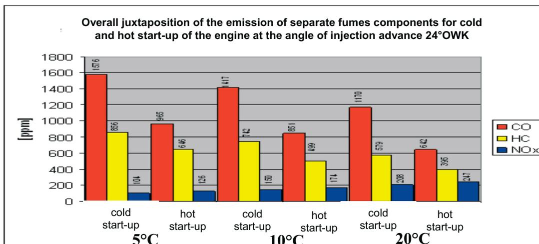
Fig. 8. Overall juxtaposition of the emission of separate fumes components for cold and hot start-up of the engine at the angle of injection advance 24°OWK
