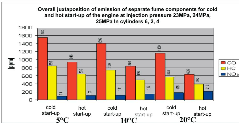
Fig. 12. Overall juxtaposition of emission of separate fume components for cold and hot start-up of the engine at injection pressure 23 MPa, 24 MPa, 25 MPa In cylinders 6, 2, 4
