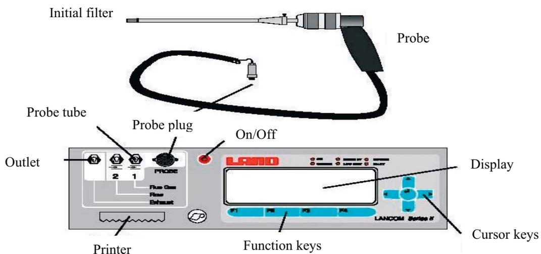
Fig. 3. General image of fume analyzer LANCOSM with fume acquisition probe
