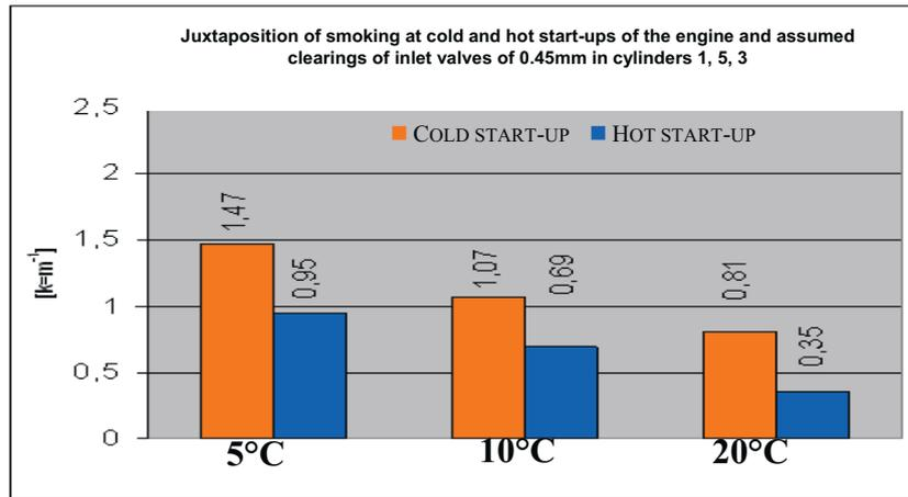
Fig. 17. Juxtaposition of smoking at cold and hot start-ups of the engine and assumed clearings of inlet valves of 0.45 mm in cylinders 1, 5, 3
