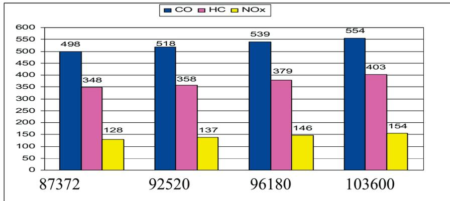
Fig. 18. Overall values of CO, HC, NO<sub>x</sub> emissions in relation to run km
