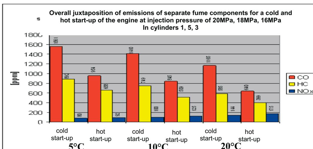
Fig. 10. Overall juxtaposition of emissions of separate fume components for a cold and hot start-up of the engine at injection pressure of 20 MPa, 18 MPa, 16 MPa In cylinders 1, 5, 3
