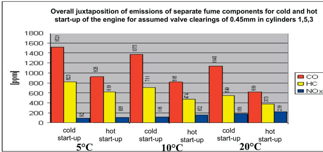
Fig. 16. Overall juxtaposition of emissions of separate fume components for cold and hot start-up of the engine for assumed valve clearings of 0.45 mm in cylinders 1, 5, 3
