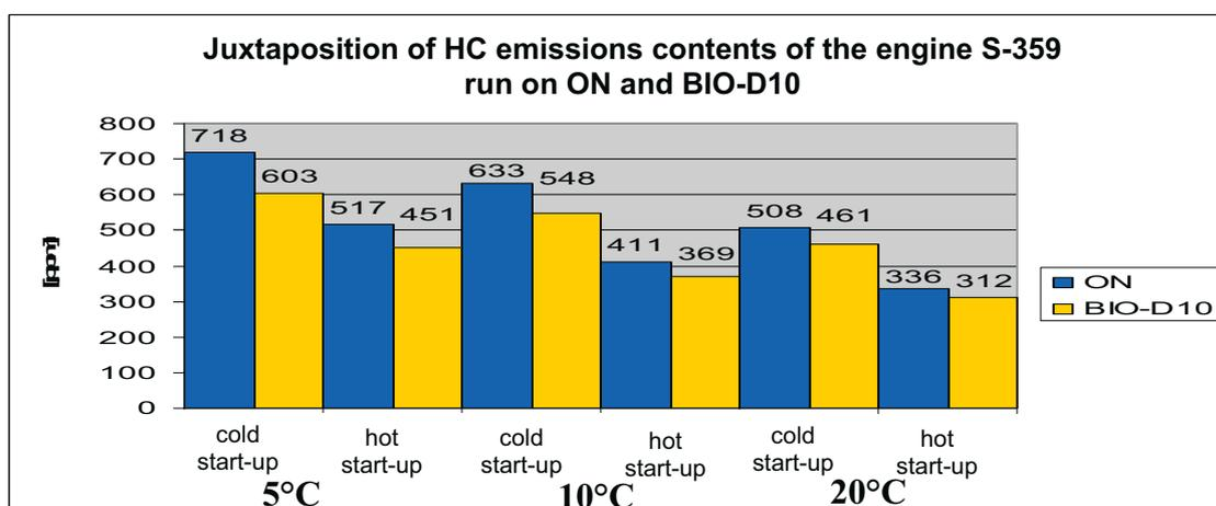
Fig. 21. Juxtaposition of HC emissions contents of the engine S-359 run on ON and BIO-D10
