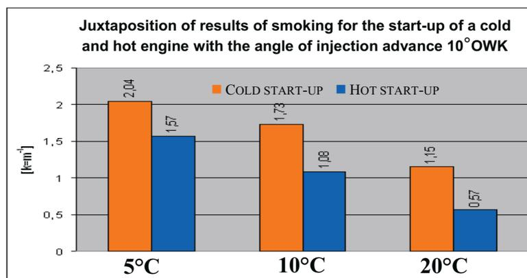
Fig. 7. Juxtaposition of results of smoking for the start-up of a cold and hot engine with the angle of injection advance 10°OWK
